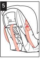
When LATCH is not being used, fasten LATCH hooks on side of child restraint as shown.
